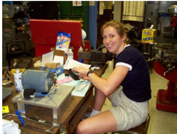
MIDN Justis attaching the strain gages to the beams.
