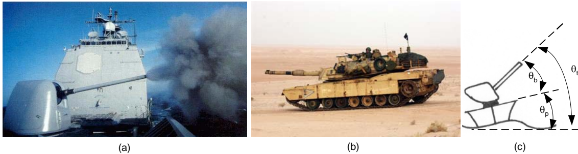
Figure 1: The Mark 45 5 inch gun (a) and M1A2 Main Battle Tank (b) both have stabilized gun barrels. The relationship between barrel elevation, platform roll, and total elevation angles (c).
