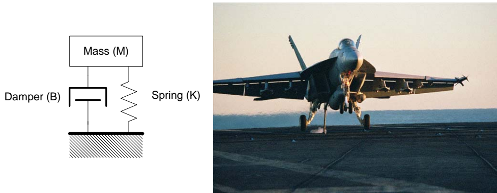
Figure 1: The spring mass damper model of an F/A-18 landing gear.
