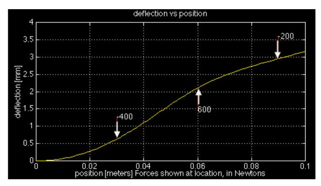
On the deflection plot the red lines are at the point of force application and they are "pushing" the beam (e.i. a positive force will have its red line below the beam "pushing" up). The values of each force is displayed at the end of its force line.
